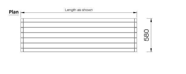
similar) western red cedar. Fitted to 3 Nr. 150x3mm metal frame @ 484mm c/c. Metal frame bolted to suitable concrete base or country kerb at regular intervals (max 1.5m distance)
